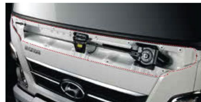
Detachable upper front panel The detachable design allows for quick inspections and easier servicing.
