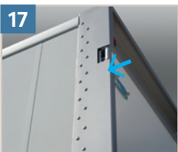
Rear door frame fastened with mono rivets
